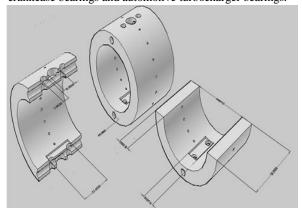
Fig: 1. Hydrodynamic Twin Groove Journal Bearing
