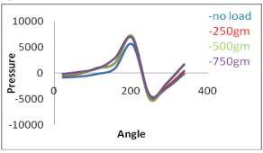
From the graphs it is concluded that the pressure profile follow the same pattern as followed by the single groove bearing and as the load increases the pressure also increases. Maximum pressure obtained for 750gm load for lubricant 15w40.
