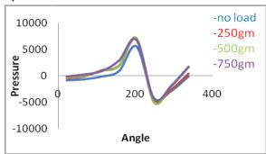
Rpm-1120, lubricant-Refined oil
