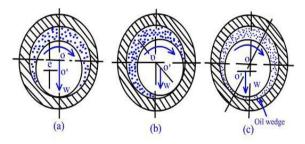
Fig: 2. Operation of Journal Bearing: (a) Rest (b) Low Speed (c) High Speed
